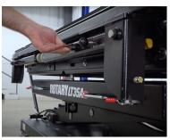
Adjustable feet on each leg table can be raised or lowered to level the table surface.
