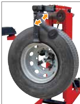
STANDARD ROLLER for tubeless tires
