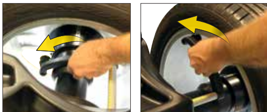
Quick selection and rim run-out measurement with internal data gauge.
